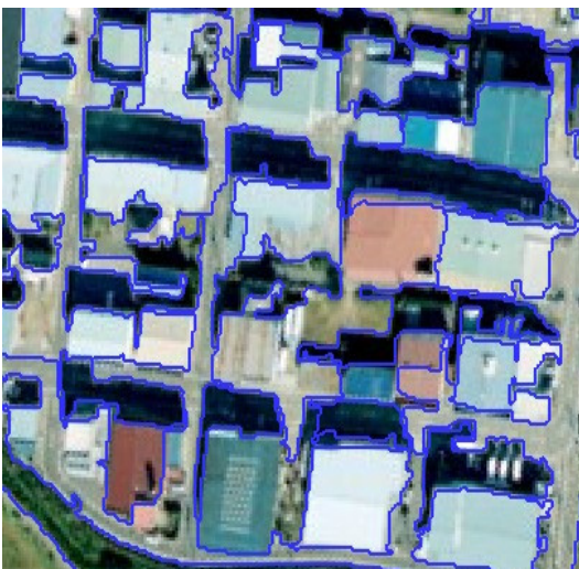
Figure 2 Building contours extracted from aerial photo by pattern recognition software (eCognition, Definiens Inc.)
